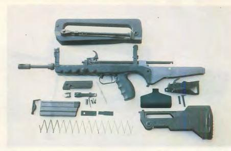
rate of right-hand twist remains one turn in every 12 inches. An optional pitch of one turn in 9 inches is available as a compromise to accommodate the SS 109 projectile. But in spite of its compactness, the FA MAS weighs 8.0 lbs. empty and minus the bipod — at the outer limits by today's standards. Steel parts are phosphate finished and the receiver has been anodized gray.
